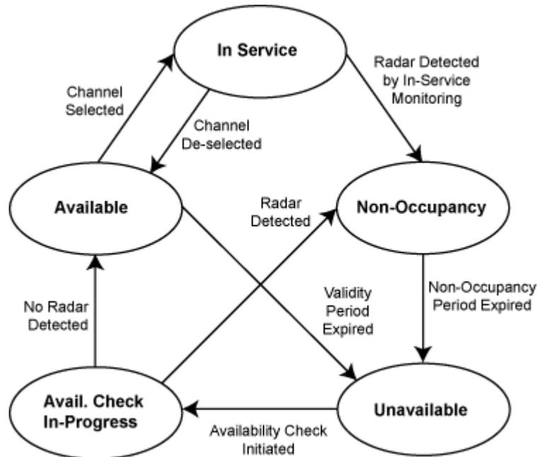
Figure 1 - DFS channel state transition diagram
